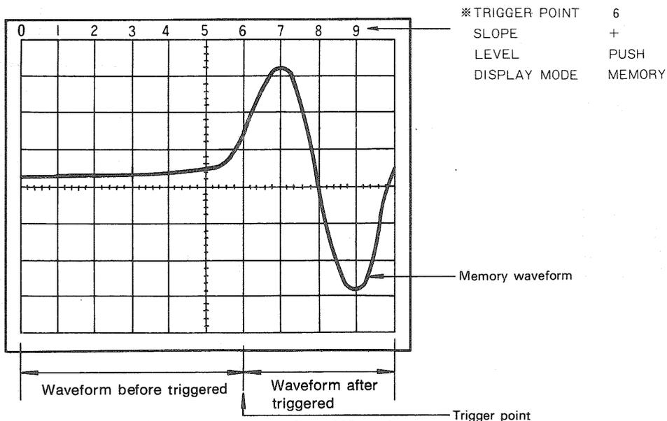
The left 6 div waveform is a memory waveform (600 words) before triggered. The right 4 div waveform is a memory wave (400 words) after triggered.
