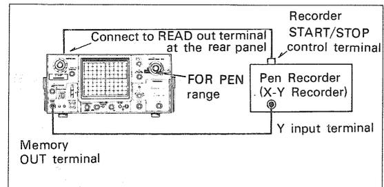
Fig. 5. Data recording with pen recorder
