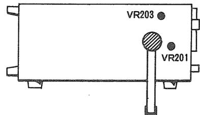
Fig. 26 DC BAL adjustment
