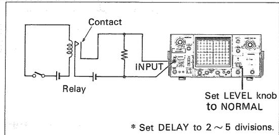
Fig. 4. Measurement of relay chattering
