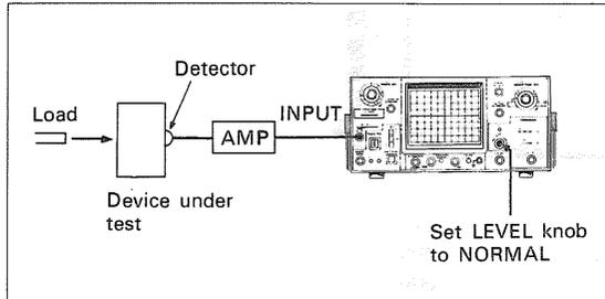
Fig. 3. Memorizing the transient phenomenon of mechanical impact waveforms
